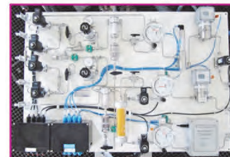
AEL-Demonstrator Measurement System for H 2 & O 2 with SIL2-Approval
