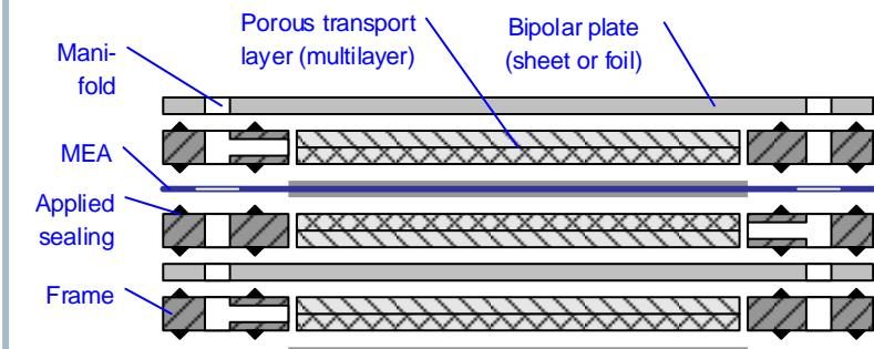
Ti foil as bipolar plate w/o channels but with Ti spacers
