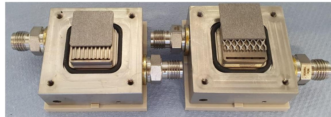
Different cell configurations with PTLs, spacers and flow fields (© Fraunhofer ISE)
