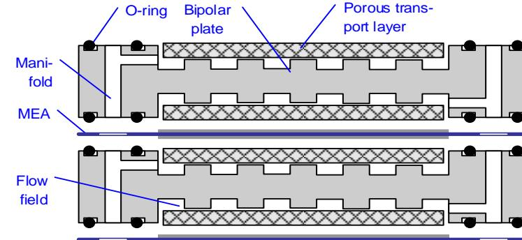
Ti sheet/foil as bipolar plate without flow channels
