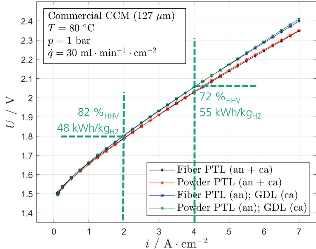
Polarization curve of different PTL setups measured with Fraunhofer ISE laboratory reference cell
