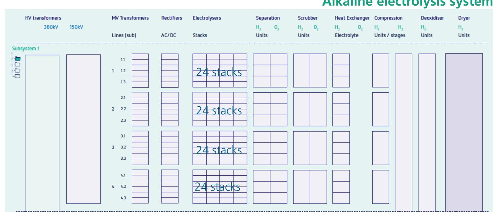
Modular design of a state-of-the-art 1 GW green hydrogen plant based on alkaline technology
